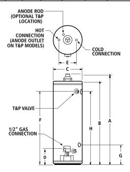
Maximum Hydrostatic Working Pressure: 150 PSI
