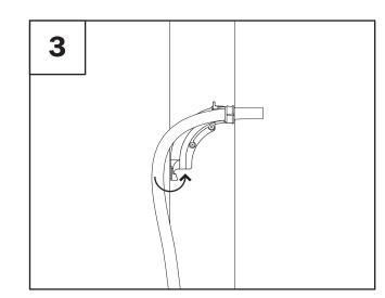
Holding opposite end of tube, guide tube through radius and around small hook on 'tail' end of the bend support.
