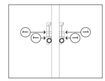
Two plastic elbows may be installed to straddle a stud for hot and cold supply.
