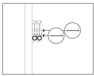
Using longer screws, two plastic elbows may be stacked against one side of the stud.
