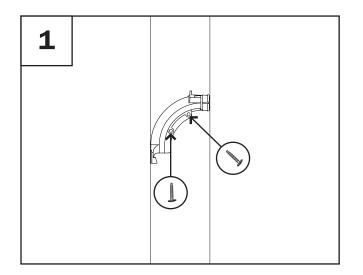
Using nails or screws, install plastic elbow directly to stud.
