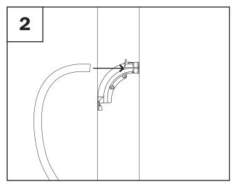
Insert end of tube into top 'nose' of plastic bend support.
