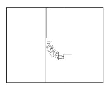
Plastic elbow may be installed on either side of stud, with flexible supply tube from above or below.
