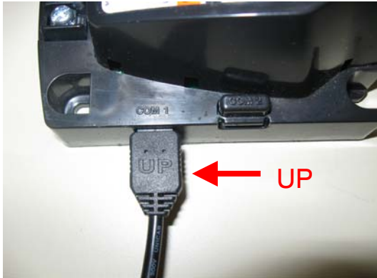
Figure 3 Tool cord set in COM port 1 with "UP" toward top of control
