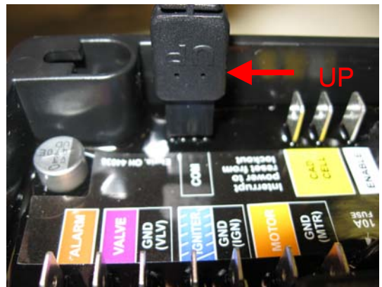
Figure 6 Tool inserted into 12VDC control COM port with "UP" towards the terminals
