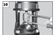
Using a screwdriver, lift the Shaft to its full travel upward, then lower half the distance and tighten and torque the Coupling Bolts.
