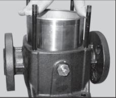
Spray soapy water on the Sleeve O-rings (Pos. 37). Then lower and press Sleeve (Pos. 55) firmly into place.
