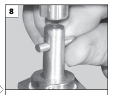
Place the Shaft Pin (Pos. 10) into the Shaft (Pos. 51).
