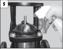
Spray soapy water onto the Seal O-ring Seating Surface of the Pump Head and the Shaft (Pos. 51).
