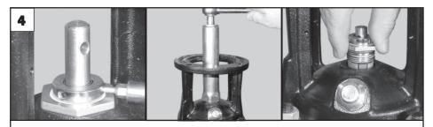
Remove the cartridge Shaft Seal (Pos. 105) by:
