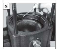
Remove, check, and replace damaged Sleeve O-rings (Pos. 37) in the Motor Stool (Pos. 2) or Pump Head (Pos. 77) and the Pump Housing (Pos. 6).
