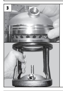
Spray soapy water on the Sleeve O-rings (Pos. 37) in the Motor Stool or CR(I/N) Pump Head. Then lower and fully press in place. For I/N models, place the Motor Stool Bracket (Pos. 2) over the Pump Head and press against this to seat the Pump Head.
