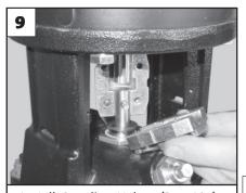
Install Coupling Halves (Pos. 10a). Spray a light machinery oil onto the Coupling Bolts (Pos. 9). Install loosely into the Couplings.
