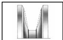
Worn Groove Sidewalls
