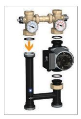
3. Rotate the connecting pipe 180° relative to its axis.
