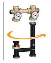
With UPS 15-58 pump the electronic housing of the pump must be removed by unscrewing the four screws indicated by the arrows and turning the body 90° counterclockwise and reinstalling. Without performing this task, it is not possible to push the group into the insulation. The ALPHA 25-55U pump will fit inside the insulation without any modifications.
