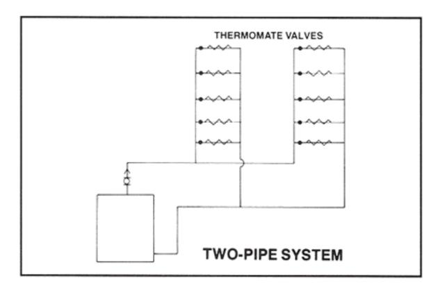
They don't work well on loop systems (unless you modify the system) because when the valve in the first room on the loop closes, the water flow to every other room on the loop stops as well.
