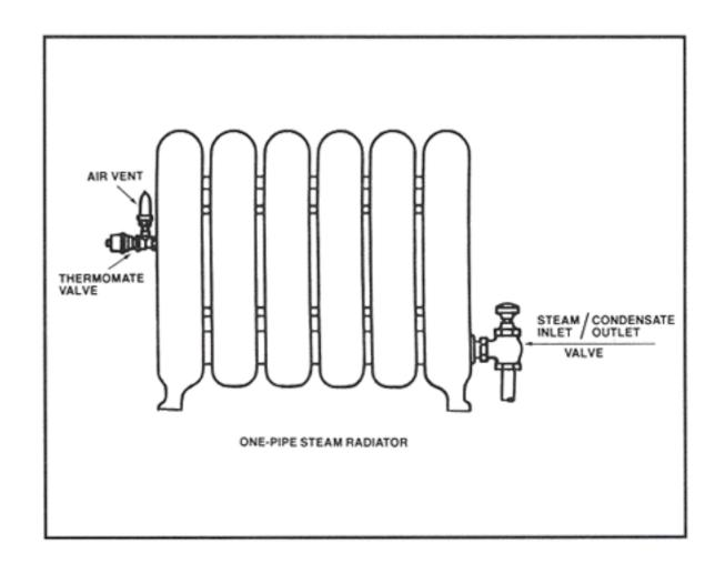
You install the valve between the radiator and the air vent. Normally, the ThermoMate's valve body is spring-loaded open. On start-up, the steam system doesn't even know it's there. Air just vents out of the radiators as it normally would.
