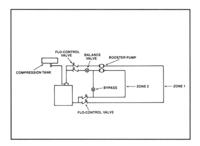
We use a full-size bypass line with a full-port balancing valve. We also have a thermometer on the discharge side of the circulator. When we start the zone circulator, all the system water will flow through the bypass because that's the path of least resistance.
