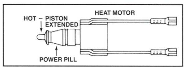
The piston pushes against the spring-loaded lever that normally holds the valve closed. This action lifts the valve disc off its seat and opens Comfort-Trol's valve. Water now has access to the zone. But remember, nothing is flowing yet because the circulator (Pumpman!) hasn't yet been called on by the Comfort-Trol valve.
