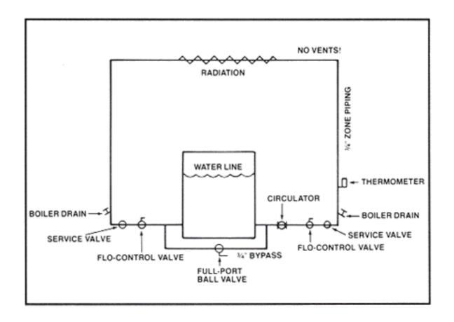
We run a continuous 3/4" loop from the boiler up through the baseboard on, say, the third floor. From there, it returns to a point on the opposite side of the boiler. Naturally, both of those connections *must* be made below the boiler water line, as low as possible, but not in the mud leg. This system is much easier to pipe on a cast-iron boiler than it is on a steel boiler because there are more tappings on a cast-iron boiler.
