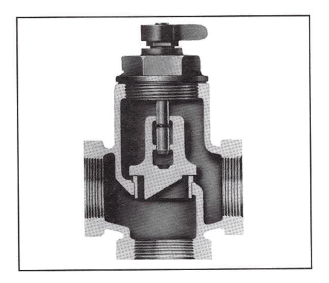
What we have inside is a brass weight that's loosely connected to a stem. The weight normally sits in the closed position and keeps the lighter hot water from rising out of the boiler when the circulator's off.
