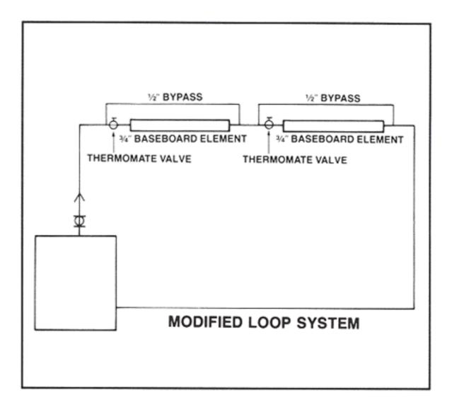
As each ThermoMate valve closes, the water will bypass through the ½" line and flow to the next radiator. When the ThermoMate valve is open, water will flow through the fin tube because that's the path of least resistance.
