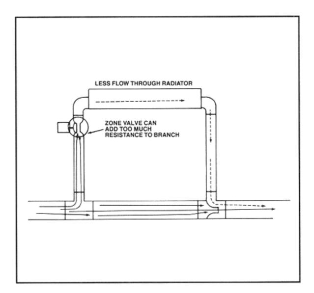
This is where it gets tricky because you can easily stop all flow to the radiator. It's like adding a second jackknifed tractor trailer to the mix. But this one's on the service road!
