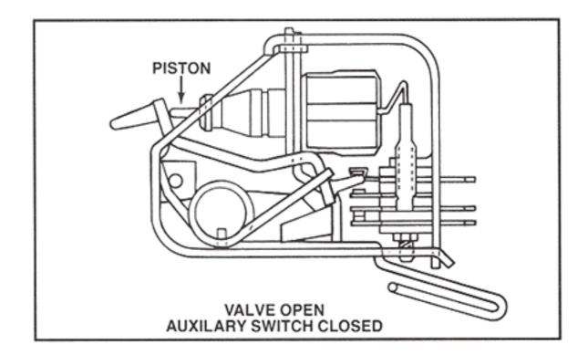
The end switch makes a connection (through a relay) back to the circulator. The circulator instantly comes on and moves water through the Comfort-Trol valve and out to the radiators. (In systems without tankless coils or side-arm heaters, the end switch, working through the relay, would fire the burner at the same time it starts the circulator.)
