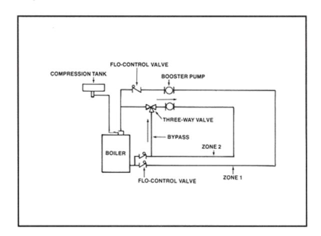
This is how commercial systems work. The 3-way valve senses what's flowing out to the system and adjusts the zone supply temperature as needed.
