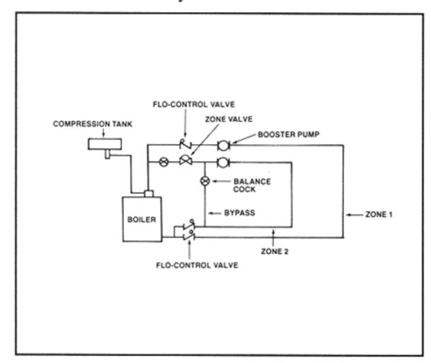
This does the same thing as the three way valve but it does it with a standard 2-way zone valve. The control sequence can be the same as what we talked about for the 3-way valve.
