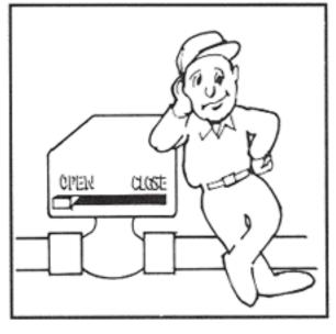
When one of the Gate Keepers is told by a Heatmaster to open a valve, water will have access to that zone. But please understand that it won't flow yet. It just has access to the zone. Nothing flows without ... Pumpman.
