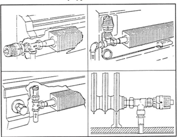
As you can see, the control knob can be either builtin or remote. So can the sensor.
