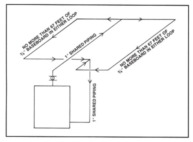
The Btuh/foot rating on ½" and ¾" is the same, by the way, because the smaller pipe allows for more fin area. Notice, however, that the total allowable length of the run is much shorter with the ½" baseboard. That's because you get a lot less water through the ½" pipe.
