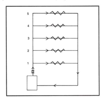
We call this a two-pipe, direct-return system. "Direct return" comes from the fact that the first radiator supplied with water is also the first radiator to return its water to the boiler. The water returns...directly. Get it?
