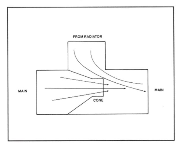
That cone restricts the water that's flowing through the main. From the water's point of view, it looks like a jack knifed tractor trailer laying across a couple of lanes on the highway. To avoid the traffic back-up in the main, some of the water jumps onto the "service road" — the pipe going to the radiator.
