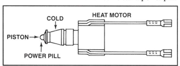
The power pill is filled with a temperature-sensitive wax that expands when the heat from the heat motor hits it. As the wax expand, it pushes a piston out of the power pill.
