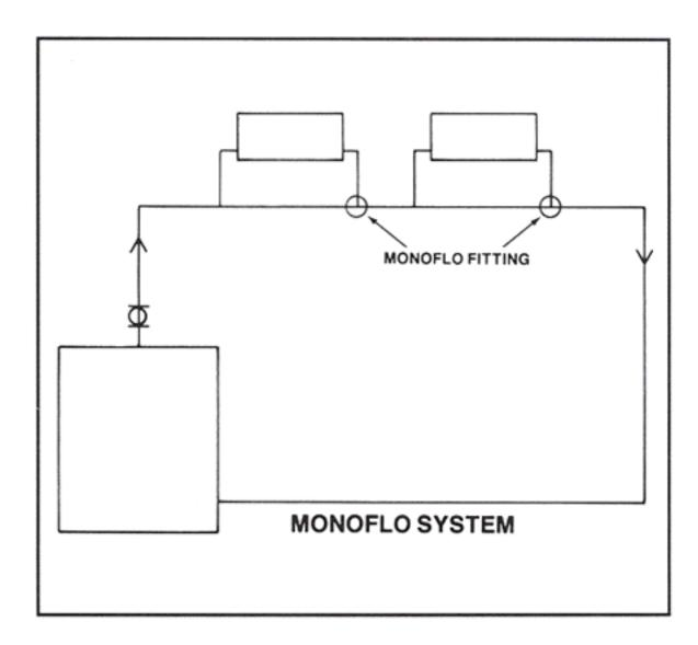
A Monoflo system is a one-pipe system. The supply and return to and from each radiator is carried by a single main.
