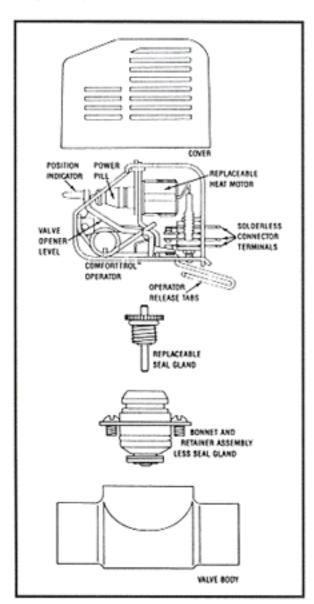
This is Bell & Gossett's Comfort-Trol® zone valve. It comes in two parts: the valve body and the operator.
