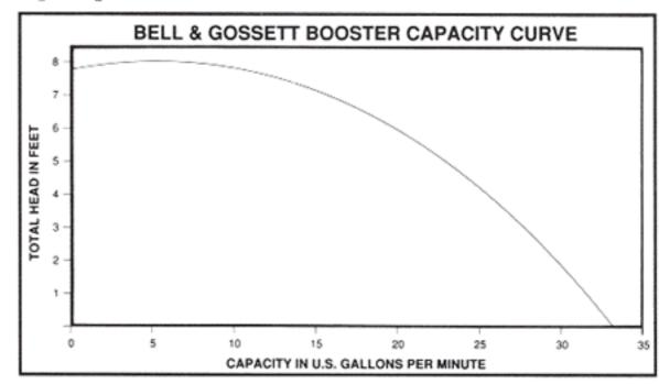
This is the performance curve for the Series 100. It's sort of like a "fingerprint" for this particular circulator.
