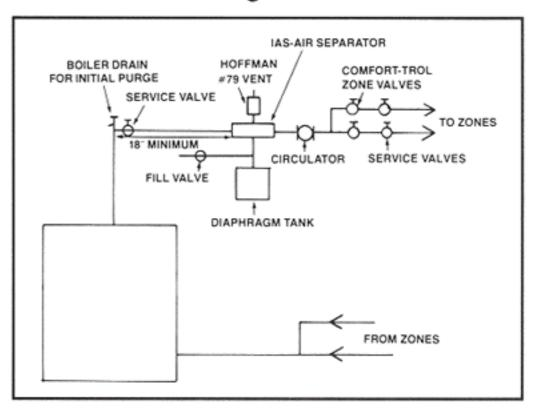
and have all the components between isolating valves.
