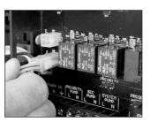
Feed wiring through hole near the top of the transformer and insert transformer plug into the socket.
