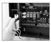
Slide bottom end of transformer into bottom latch.
