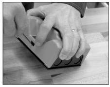
Hold either the left or the right end of the box up and at an angle. Use body for stabilizing relay box. Insert screwdriver and push tab inward.
