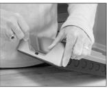
Hold either the left or the right end of the box up and at an angle. Use body for stabilizing relay box.
