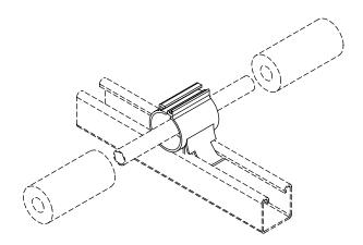
THE HOLDRITE® Insulation Coupling "8 Series" clamps are designed for use with insulated pipe lines mounted on strut. These one piece clamps are non-metallic and fasten simply with the use of a pair of pliers and without any hardware or fasteners. Recommended for horizontal positioning only.
