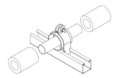
THE HOLDRITE<sup>®</sup> Insulation Coupling "7 Series" strut clamps are for use with insulated pipe lines mounted to strut in any orientation. These are plenum rated insulation clamps are ideal for insulated pipe line support without the need for rigid insulation supports or insulation shields.
