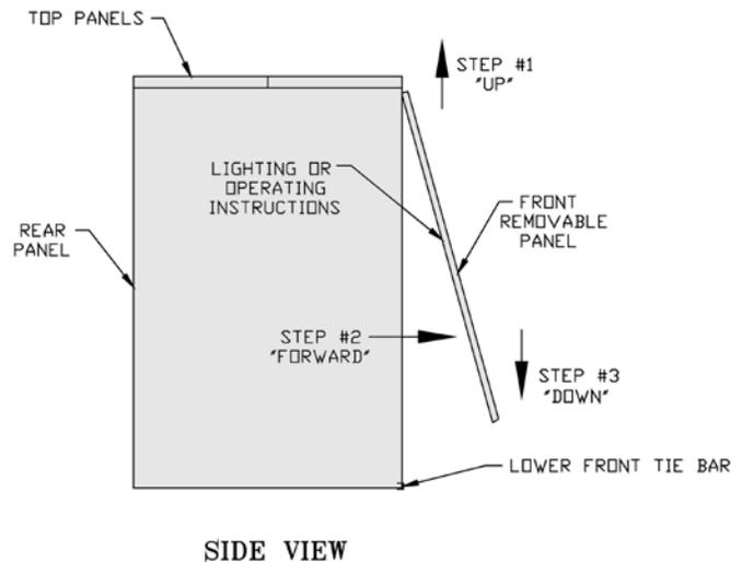
**Figure 3: Jacket Front Panel Removal**
