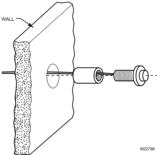
Fig. 18. Mounting sensor in wall with spacer only.
