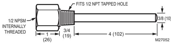
**Fig. 2. 50001774-001 Immersion Well dimensions in in. (mm)**
