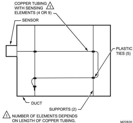
Fig. 12. Duct cross section showing method of installing C7041R Averaging Electronic Sensor.
