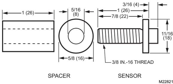
**Fig. 3. Dimensions of the C7041P in in. (mm)**
