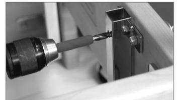
Figure J: Rubber bumper prevents you from drilling into frame too far. Drill
