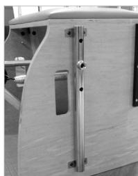
3. Install two 7/8" buttonhead screw and washer assemblies into the two holes of the lower receiver tab. Push the screws through the wooden side of the chair and use the allen wrench to engage the threads into the propeller nuts.
