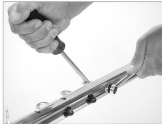
Screw the cap nut onto the eye bolt, flush with the disk. **DO NOT** overtighten the screws – this can damage the parts. **Note:** attach the push-through bar **AFTER** you have secured the Tower to the wall and floor.
