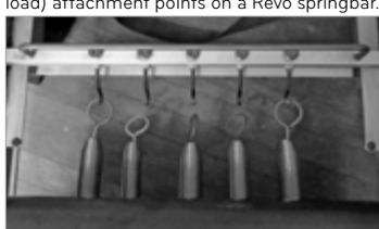
"Hook" attachment point found on Revo Springbars, Standard Springbars and some versions of the Allegro Reformer. Note the Hour Glass posts in the upper section of this springbar as a pre-load position, shown here without the springs attached.
