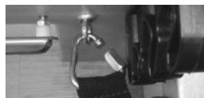
Figure 2: Good snap: no wear on hook.
