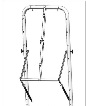
**Note:** Use the velcro portion of the safety strap oriented at the top of the tower frame to secure the PTB upright when not in use.
