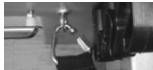
Figure 2: Good snap: no wear on hook.
