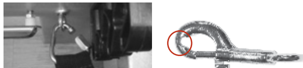
Figure 2: Good snap: no wear on hook.
