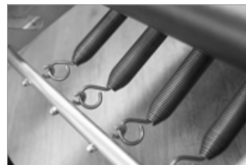
"Hook" attachment point found on Contrology Reformers.
