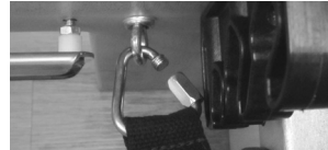
Figure 2: Good snap: no wear on hook.
