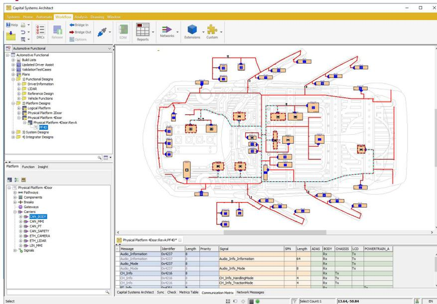
Capital Systems Architect can help visualize networks within a platform and provides support for signal and message mapping
