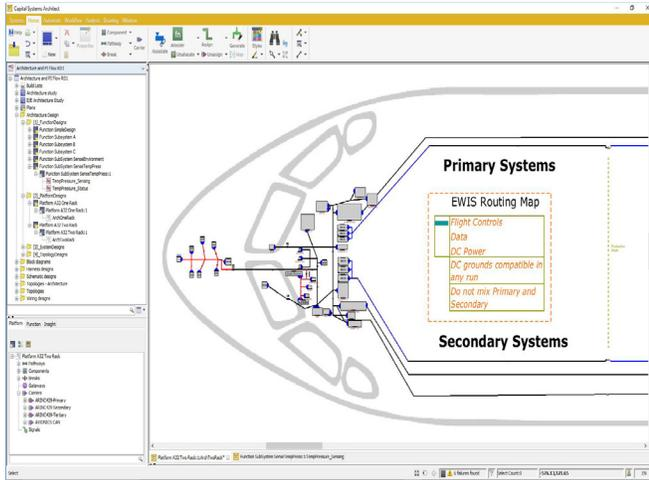
*Functions and signals can be assigned to components and carriers allowing engineers to build a platform architecture to help optimize decision making early in the design process*
