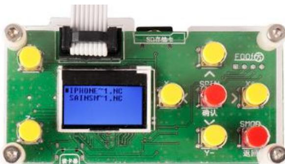
Note: The system recognizes up to 200 valid files at a time. Support for the following formats: xxx.TXT /xxx.txt /xxx. NC /xxx.nc /xxx.CNC /xxx.cnc /xxx.TAP /xxx.tap
