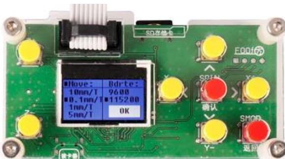
On the left is the distance that the machine moves after each button press. Press Y+ or Y- to select.
