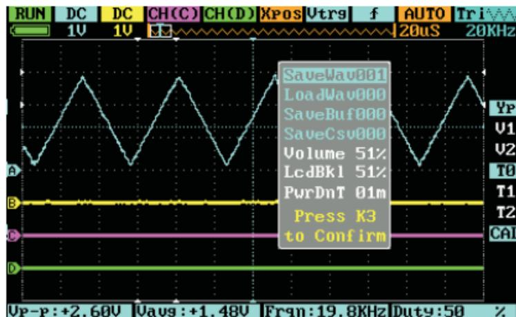
2) Input waveform signals that are to be compared in Channel A, select "REC\_A" in position E, press button "●" to select "LoadWav001", see following picture;
