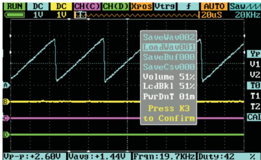
3) Move "Yp" in position K to adjust the horizontal line and then compare the waveforms.
