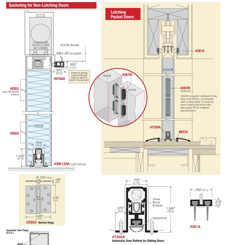
This automatic door bottom functions differently from other ZERO door bottoms. When the plunger is compressed, the mechanism causes the insert seal to activate and drop evenly along the door bottom.
