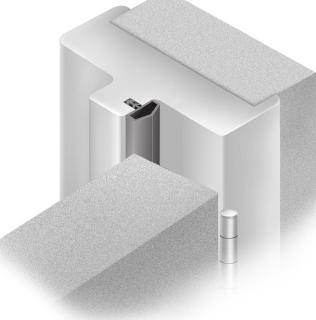
Pre-groove the jambs or stops before installation. Cut a 3/16" x 1/4" (4.7mm x 6.4mm) groove in the center of any width rebate. (See drawing for location.)
