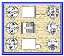
Mortise cylinders had two cams. The bottom cam had a gear that meshed with the main gears mounted on the back of the cylinder. The cam closest to the gear operated off of the top core and had a gear wedged into it. The top cam worked directly off of the bottom core.
