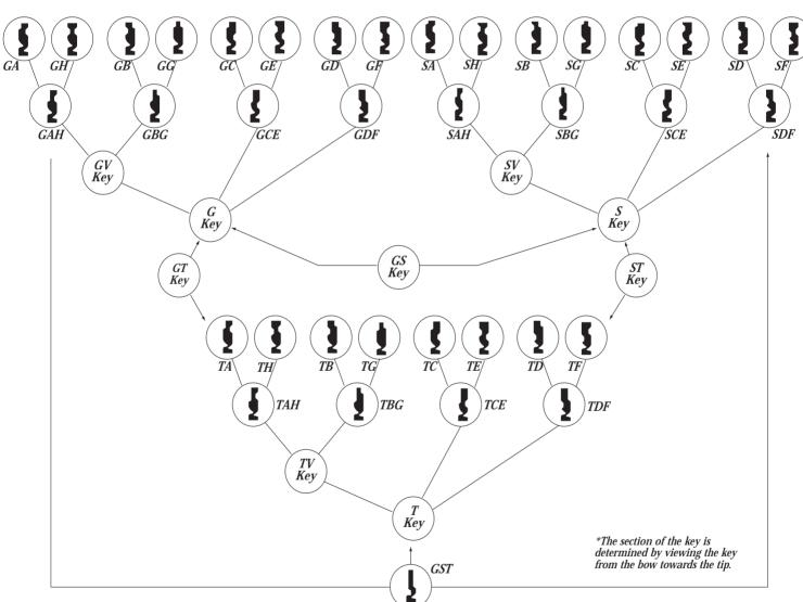
Note: Yale locks and cylinders are available with a wide range of key sections (keyways) to meet almost any keying requirement. In addition to the stock sections (PARA/E1R and the G,S and T families), there are many restricted keyways available both as simplex key sections and multiplex families. A letter of authorization from the end user may be required for the purchase of product that is restricted or keyed into an existing masterkey system. Please contact us for additional information.
