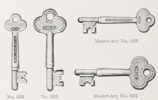
Master-keying: These locks can be master-keyed in one set of 1890 locks, all different, with a master-key to pass all locks; or in sets as desired and with other locks using master-keys from No. S55 or S50 blanks.
