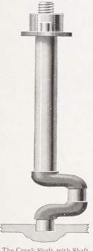
The Crank Shaft with Shaft Driver; showing Step-Bearing
