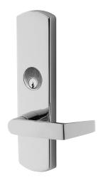
E996L Electrified lever trim provides remote locking and unlocking. Available in either fail safe (FS) or fail secure (FSE) condition, but can also be field converted where allowed. E996L is furnished standard with cylinder operation for nightlatch (NL) function, or with blank escutcheon (BE).
