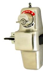
The Von Duprin Classroom Security Indicator provides an at-a-glance verification of the locked/unlocked status of the door from inside of the room. This option can be ordered as a new product or as a retrofit conversion kit to an existing 98/99 device. Indicator in Unlocked state presents a 1/2" x 1/2" metal flag (white background with black icon) at top of device head. Indicator in Locked state has no flag present.
