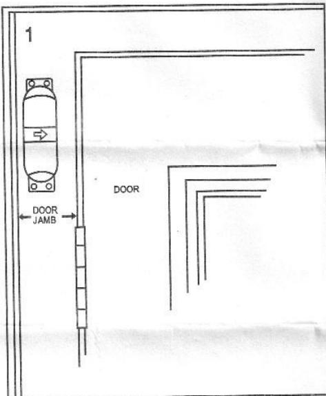
Fasten the main body of the door closer on the surface of the door jamb or door frame. The jamb or frame must be flush with the surface of the door.
