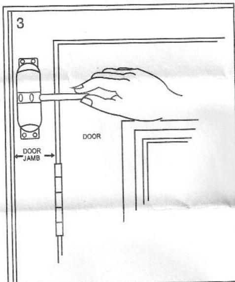
The tension regulates the closing speed of the door. To increase the closing speed, increase the tension by repeating the operation as stated in figure 2.
