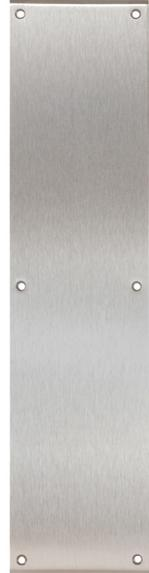
Trimco's 1001 & 1807 Series Push Plates are manufactured in the United States from .050" or .125" thick stainless steel, brass, bronze, or aluminum. All push plates are pencil or heavy beveled on all four edges and are supplied with oval head screws standard. Custom sizes and plastic push plates are also available. Options include engraving for "PUSH" or "PULL", as well as different cylinder and custom cutouts for most applications.
