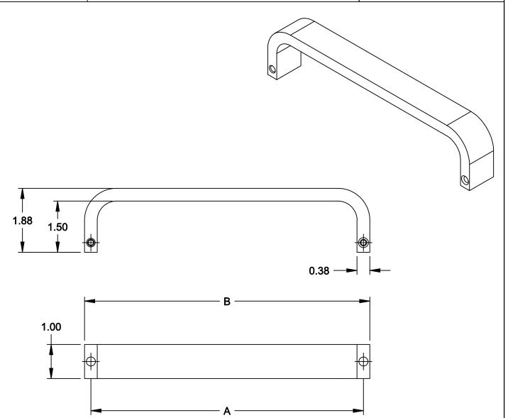
SUPPLIED WITH TWO (2) 1/4-20 SHOULDER BOLTS AND FOUR (4) 10-32 SET SCREWS
