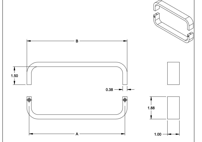
SUPPLIED WITH TWO (2) 1/4-20 SHOULDER BOLTS AND FOUR (4) 10-32 SET SCREWS
