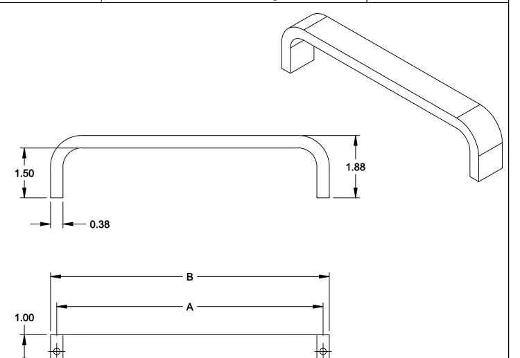
SUPPLIED WITH TWO (2) 1/4-20 FLAT HEAD, PHILIPS DRIVE MACHINE SCREWS AND TWO (2) 1/4 FINISH WASHERS.
