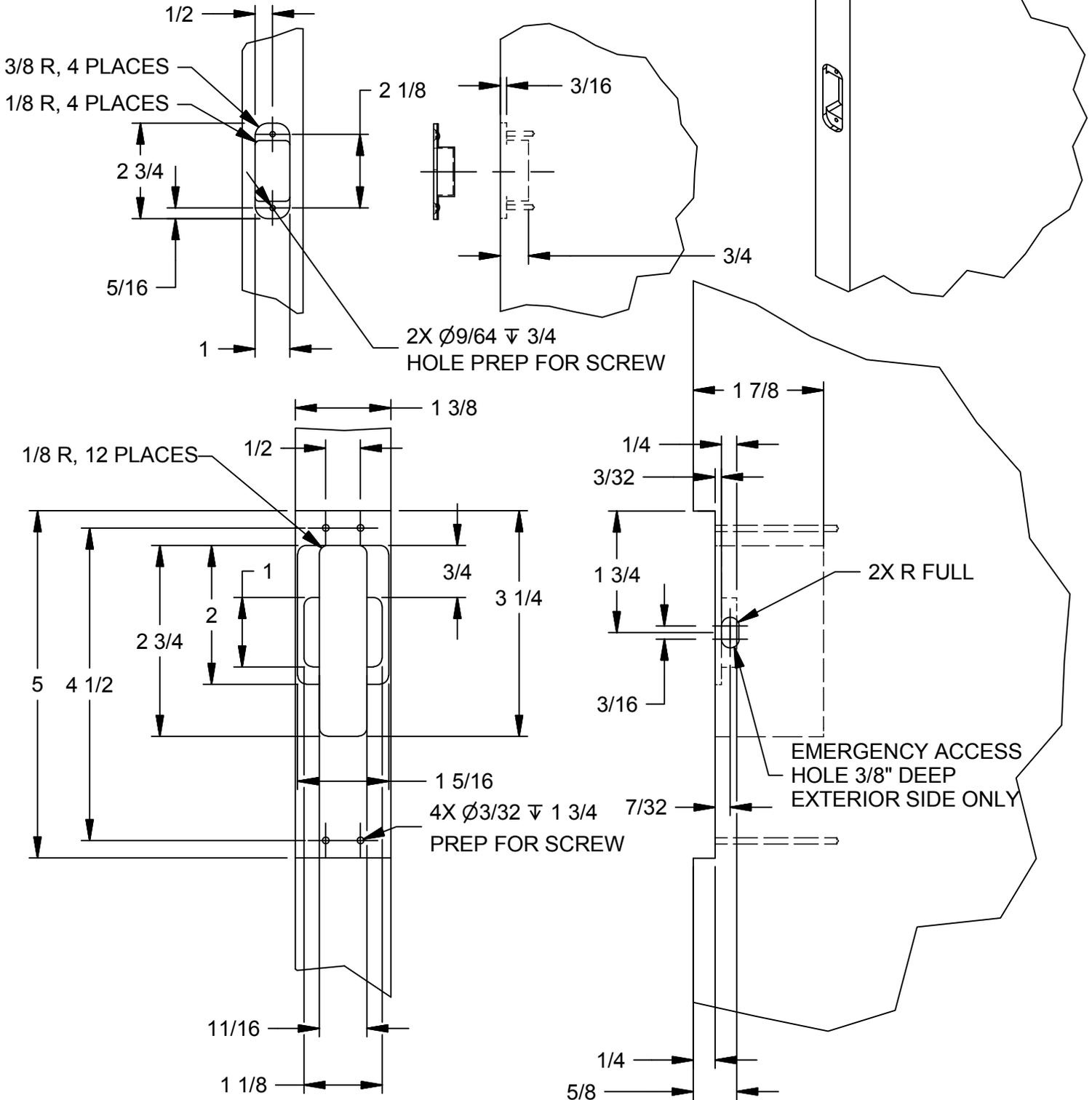
DOOR PREP FOR 1-3/8" WOOD DOOR - CENTER PATTERN IN DOOR THICKNESS
