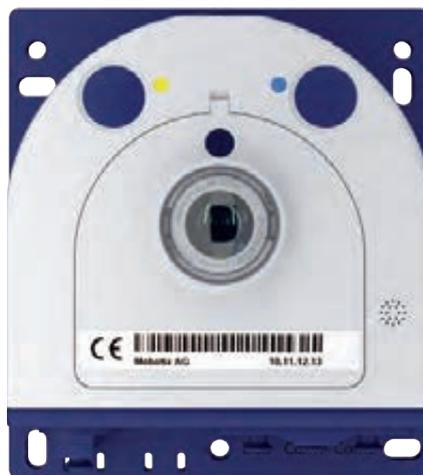
The S15M, which can be mounted discreetly behind wall or ceiling panels, is based on the S15D dual camera and thus also features weatherproof MxBus, MiniUSB and audio connectors to support various extensions.
