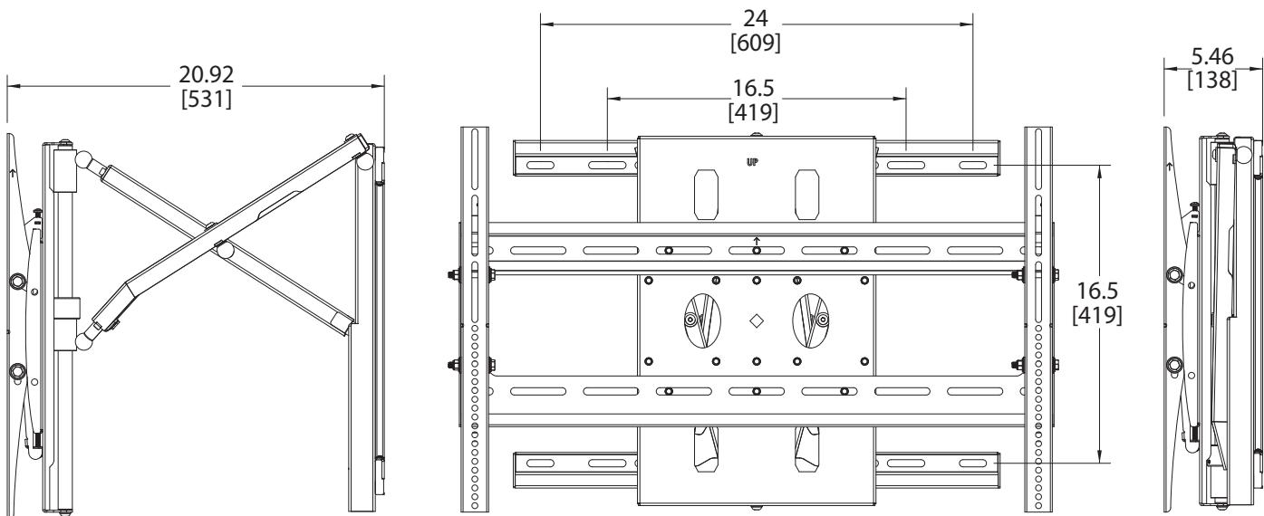
Dimensions in inches and millimeters [mm].
