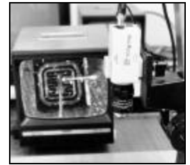
The lenses mount easily to any "C" or "CS" mount camera. An iris adjustment allows for use with inexpensive light sources.
