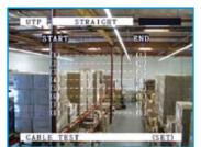
Wire map tester for UTP cabling with clear display of fault condition
