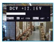
Full function digital multi-meter with large on-screen display tests AC/DC volts, AC/ DC current, ohms and continuity. Auto and manual range selections
