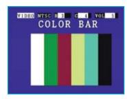
Test pattern generator outputs color bar and solid red, green, and blue screens in NTSC or PAL format
