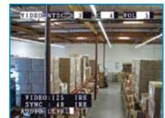
Video and sync level testing in IRE units (NTSC) or millivolts (PAL) and audio level testing with internal speaker and visible level scale. Available only in SecuriTEST PRO model.
