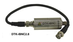
DITEK's DTK-iBNC Series inline surge protectors are designed to protect externally-mounted cameras where a dedicated ground connection is unavailable. The iBNC diverts transient surges through the coaxial shielding, protecting the video feed without introducing ground loops. Solid performance and easy installation make the DTK-iBNC Series a favorite among CCTV integrators.
