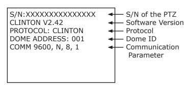
The initial information will remain on the screen until a button is pressed, joystick is moved, or until "POWER UP ACTION" initiates. See next page on how to show Initial Info within system settings menu, and how to define Power up action.
