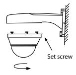
Insert PTZ tabs into mount holes and turn to lock in place
