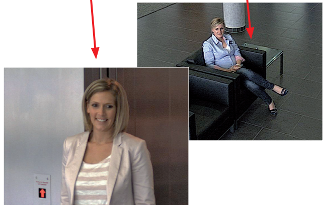
Original image: Telephoto lens (left) and wide angle lens (right) – simultaneously in one image
