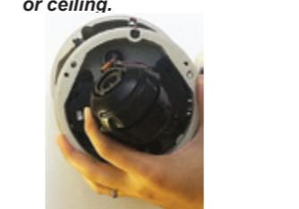
6 Snap the camera module into the base by aligning the red and black markings on the base and the camera module.
