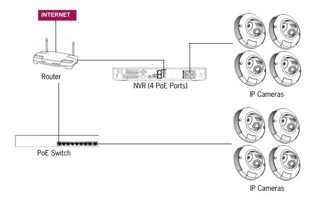
**NOTE:** Unlike DVRs, the number of channels supported on an NVR may be different than the number of physical inputs on the back panel of the unit. In the example, the NVR supports 8 channels in total. It has 4 PoE inputs for direct camera connections and can support an additional 4 cameras that are connected to the LAN, in this case via the PoE switch.
