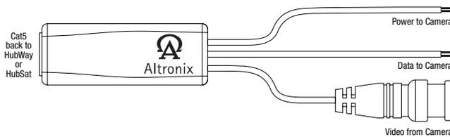
HubWayAv/HubWayAv2 passes AC voltage from pins 4, 5, 7, 8 to terminals marked [AC Power] (Fig. 3, pg. 5).
