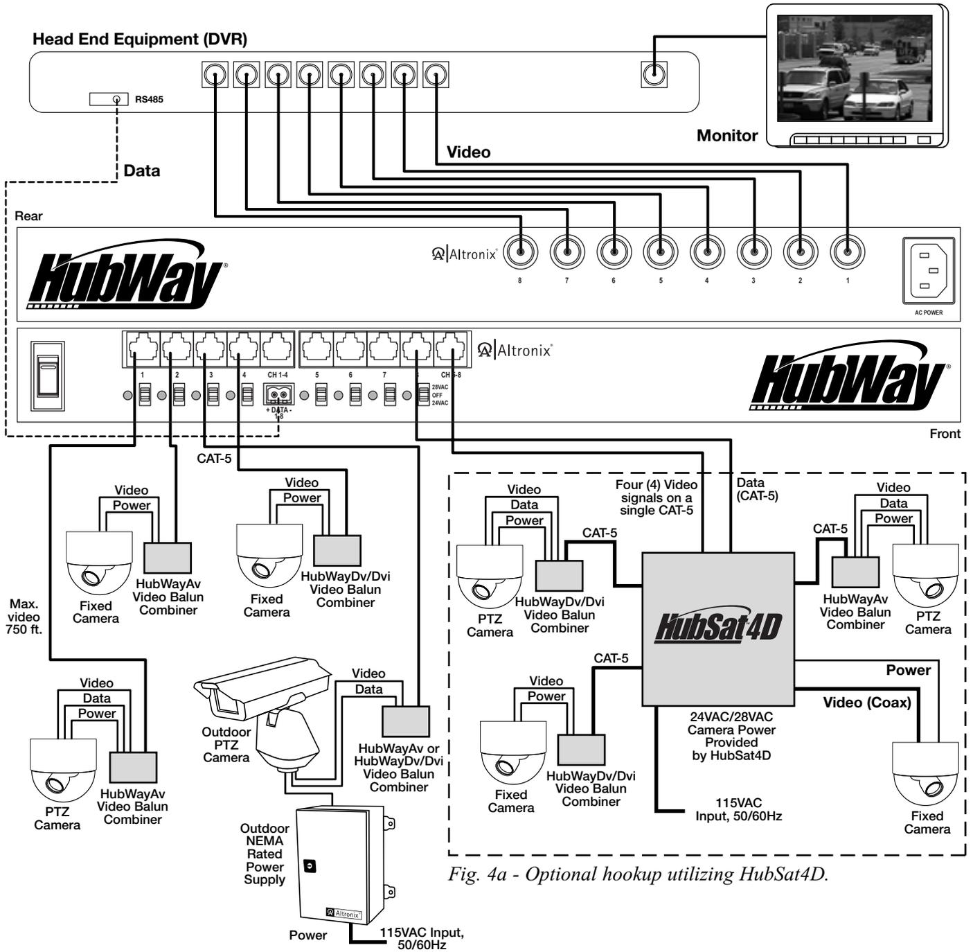
Fig. 4a - Optional hookup utilizing HubSat4D.
