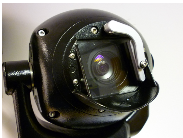
Figure 11.3: Inverted rain shield installed on camera
