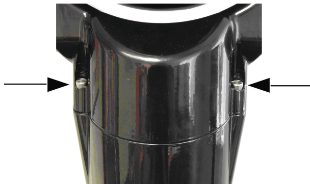
Figure 10.2: Pan body fixing screws
