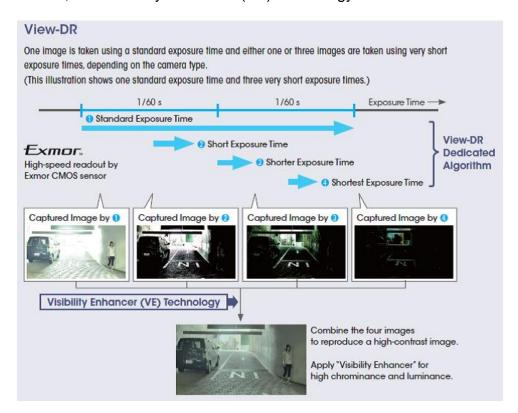
The full-capture wide dynamic range technology shall use an electronic shutter to capture multiple images and reproduce each frame.
